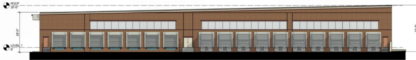
A1 WEST ELEVATION - LOADING DOCKS 1/16" = 1'-0"
