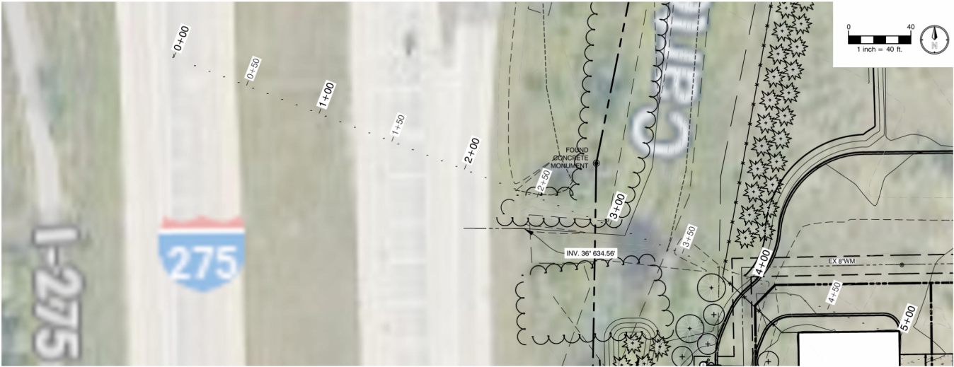
Southbound Highway Sight Lines SCALE: HORZ 1" = 40', VERT 1" = 40'
